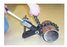
4. Take up remaining slack with knurled handle on screw. (Turn screw clockwise to tighten). As the chain is tightened, the upper jaw and lower jaw will get closer together. Make sure there is a space between the upper jaw and lower jaw chain cutter wheels when chain is snug. If there is contact between these cutter wheels, and the chain is still loose, repeat Steps 1 thru 3. Squeeze jaws as shown and hand tighten the drive screw until snug.
