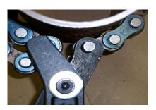
6. Once slack has been removed, place ratchet on square end of drive screw assembly. Keep turning ratchet clock wise to cut pipe.
