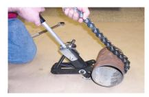
3. Pull up on inside jaw set to open cutter. (Should appear like an open pair of scissors). Choose chain pin to engage the jaw pin. Engage chain pin in pocket located on the inside of the outer jaw.
