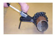
5. Once the chain is snug, make sure that the cutter wheels do not touch. At any time during the cut, if cutter wheels are too far apart, cut will result with jagged edges.
